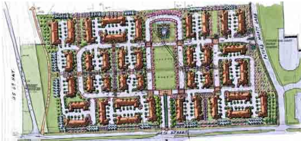
Figure 2—Multi-family buildings shall be organized around a common open space, public open space, natural features located on the site, or community amenities such as swimming pools or other recreational facilities.
