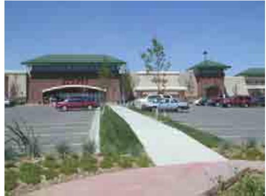
Figure 21—On-site pedestrian walkways shall connect each primary entrance of a commercial building to the adjacent parking blocks, structures, or site amenities.
