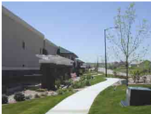
Figure 18— Each boundary to be screened between the commercial development and the adjacent use shall be landscaped with at least 4 trees and 20 shrubs per 100 linear feet of edge
