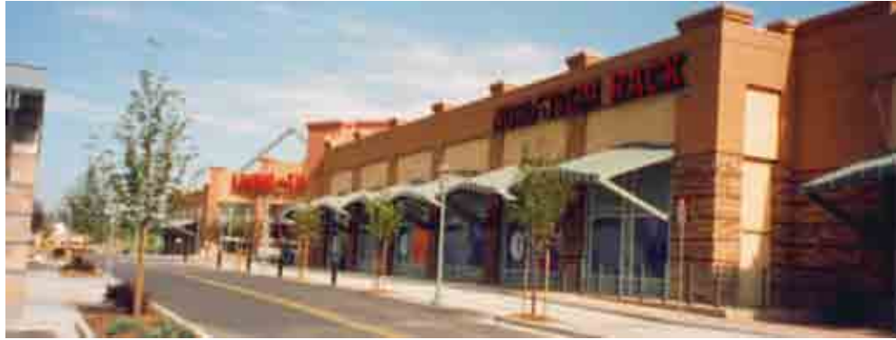
Figure 28— Facades that face public streets or adjacent development shall be subdivided and proportioned using features such as windows, entrances, arcades, arbors, awnings, trellises with vines, along no less than 60% of the façade.
