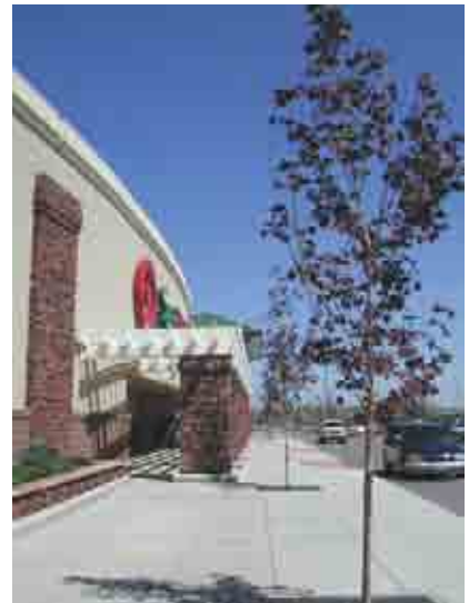
Figure 22— Continuous pedestrian walkways no less than 8 feet wide shall be provided along the full length of a primary building along any façade featuring a customer entrance and along any façade-abutting customer parking areas.
